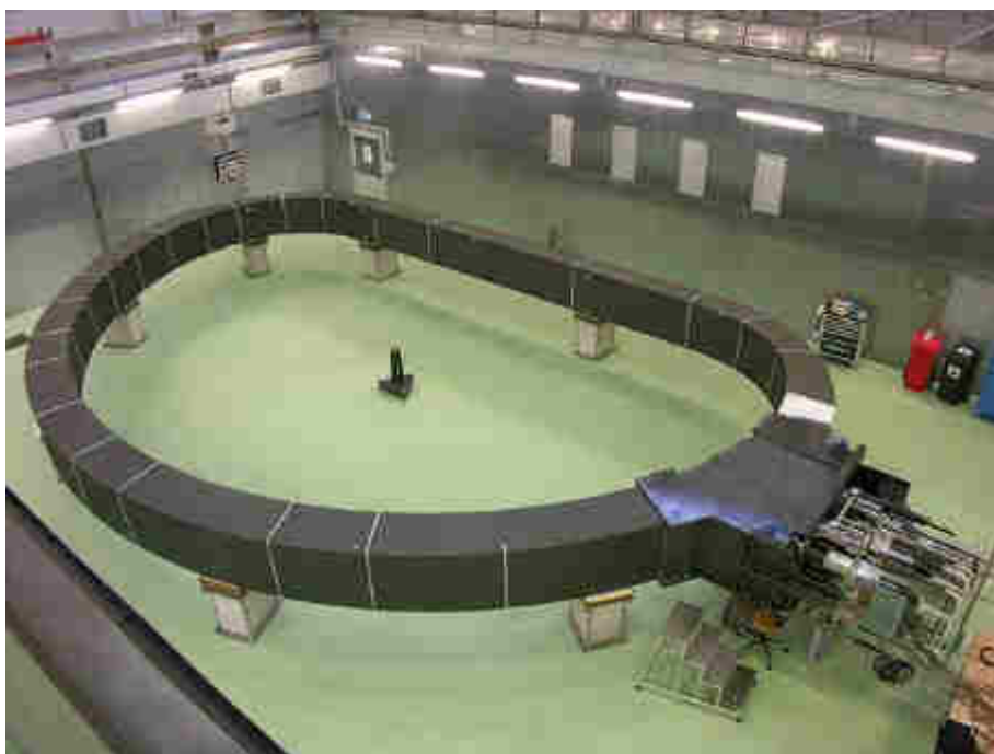
The toroidal field coil magnet - "the most high tech magnet in history", according to F4E (Image: F4E)
